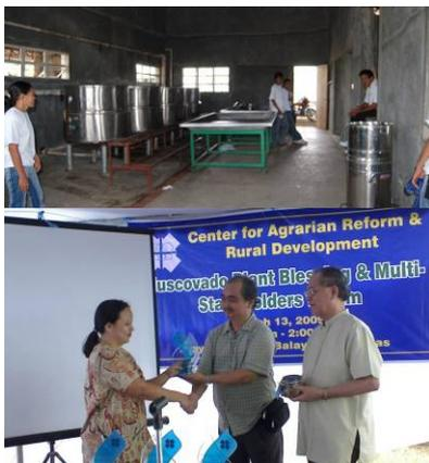
Top: The processing area showing steam fuelled boiling tanks and cooling tables;
